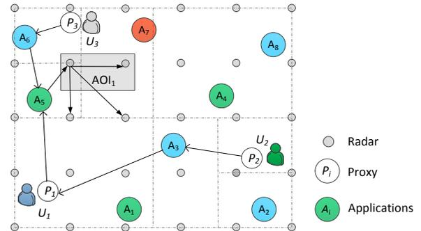
Figure 5. Named interest packet routing in a radar data fusion network.
