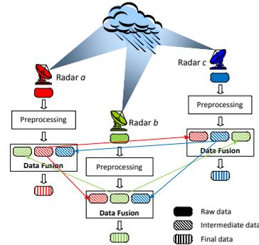
Figure 3. Radar data preprocessing and multi-radar data fusion.
