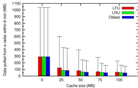
Figure 6. Data pulled from a radar under varying cache sizes and policies.
