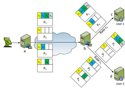
Figure 1. Application-aware packet marking and dynamic data selection.
